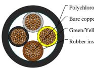
Polychloroprene rubber outer jacket Bare copper conductor Green/Yellow wire Rubber insulation
